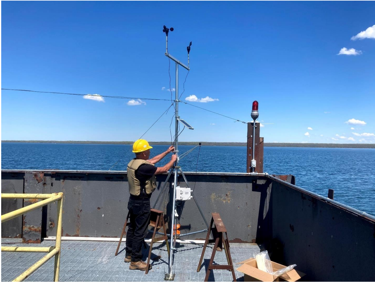
Figure 1 Meteorological station deployed at Greenidge cooling water intake structure on May 14, 2021.
