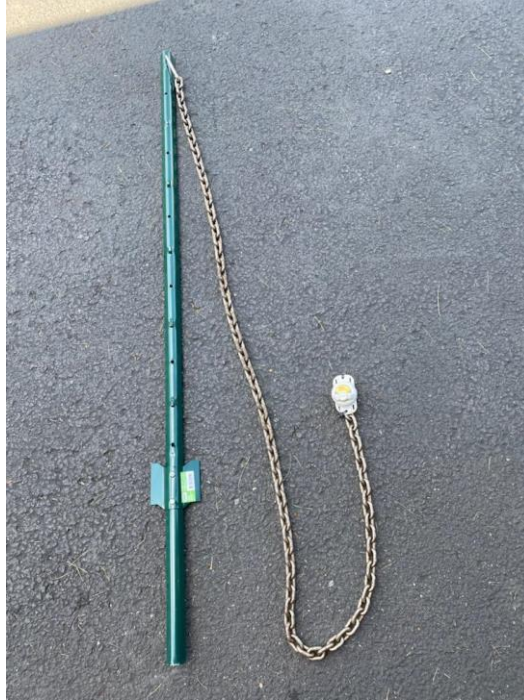
Figure 13 Stake & chain deployment apparatus for KLO stations.
